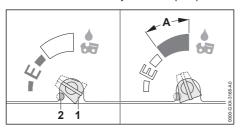
The oil feed rate is suitable for most applications when the oil pump adjusting screw (1) is in position E (Ematic).
